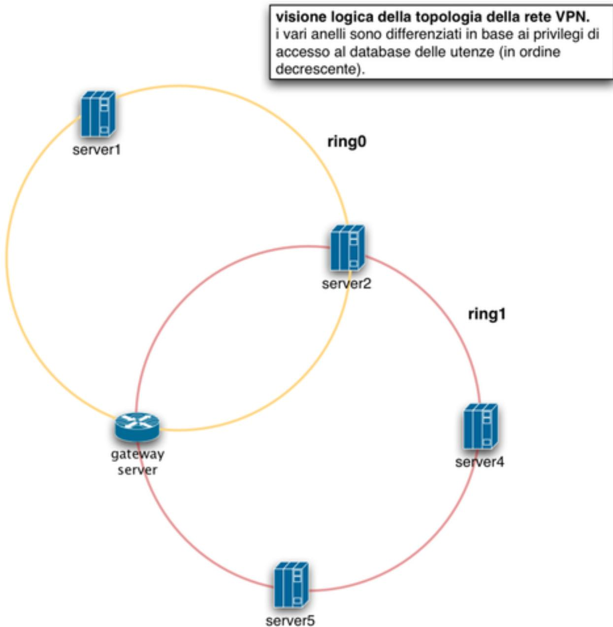
Scheme detailing the logical connection between the various servers
