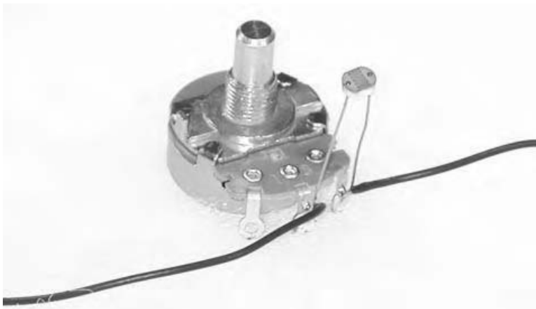
Figure 15.5 A potentiometer and photoresistor in parallel.
