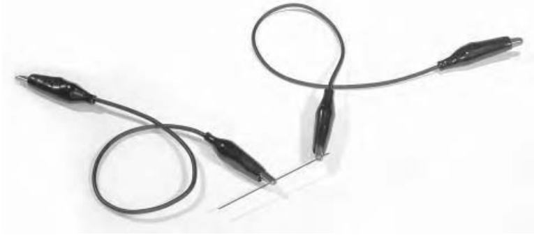
Figure 15.9 A pencil lead resistor.
