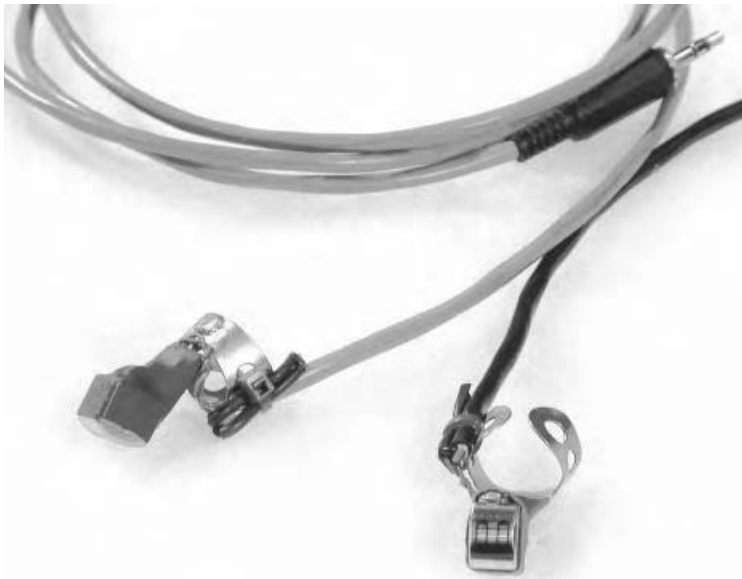
Figure 9.3 Tape heads mounted on fingerpicks, Nicolas Collins.
