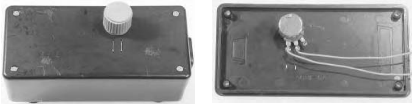
Figure 15.7 A potentiometer with electrodes in parallel.
