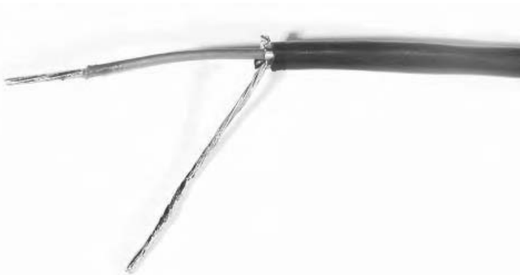
Figure 7.2 Shielded cable prepared for soldering.
