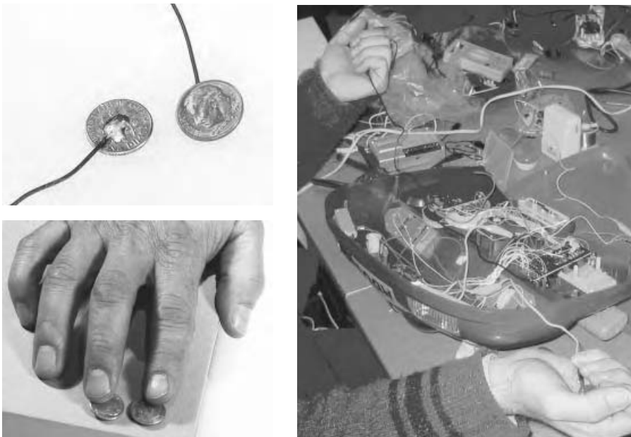
Figure 15.6 Coin electrodes and their performance.
