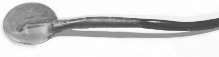
Figure 7.5 Contact mike encased in Plasti-Dip.
