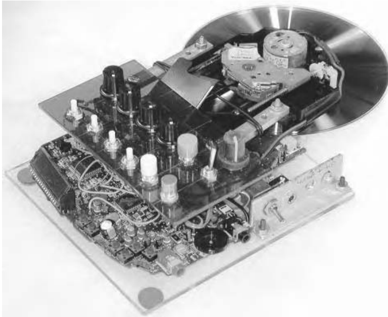
Figure 15.13 “Sled Dog,” hand-scratchable hacked CD player by Nicolas Collins.
