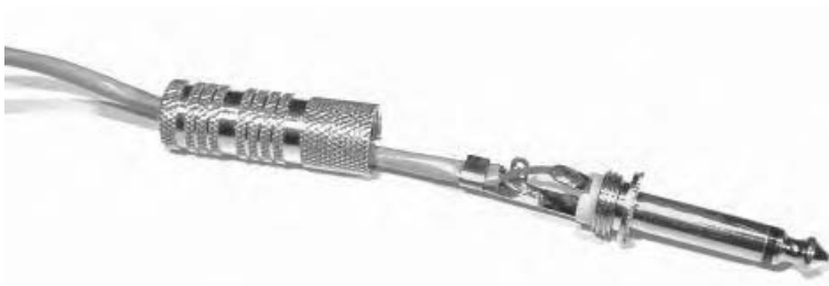
Figure 7.4 Cable soldered to plug.
