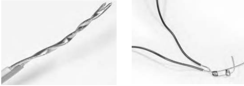
Figure 6.3 A happy solder joint (left) and a sad solder joint (right).
