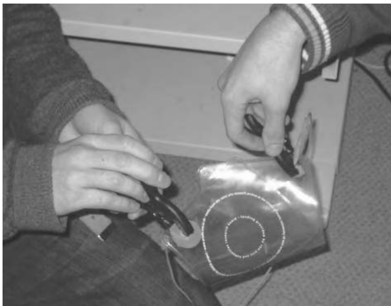
Figure 8.2 A piezo driver and contact mike pickup being used to filter a sound through a sheet of plastic.
