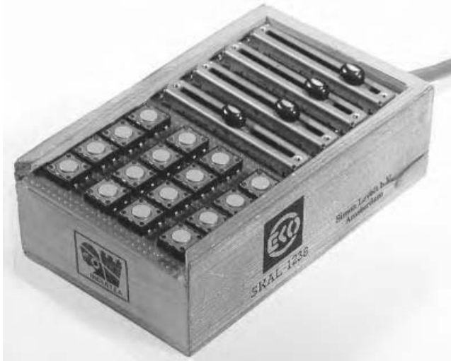
Figure 29.16 Wind controller built by Nicolas Collins from a USB interface, with four slide pots, sixteen switches, and an air pressure sensor.
