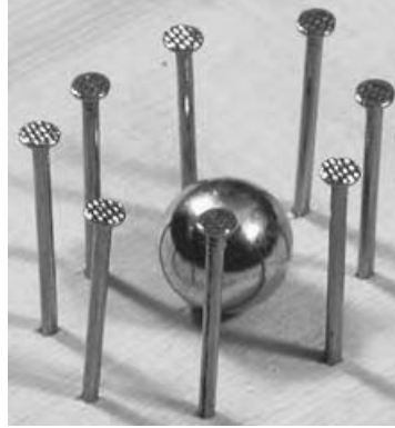
Figure 16.5 A homemade tilt switch.
